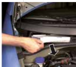
Im. 2 - Cabin filter located behind in the engine bay, under the windshield
